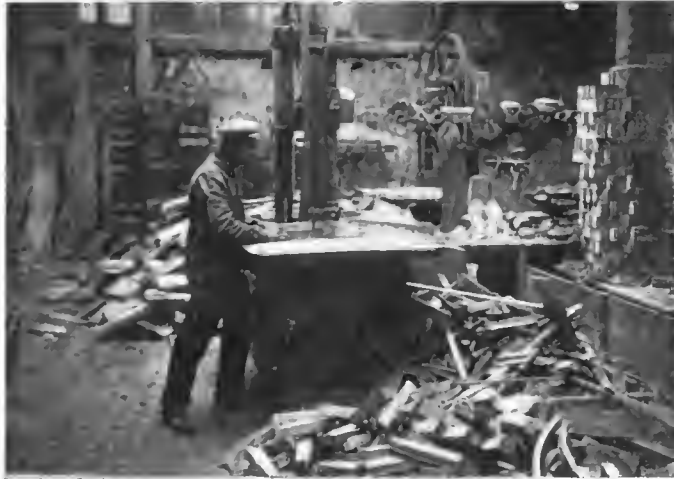
CUTTING WOOD INTO BLOCKS FOR SPOKES.
